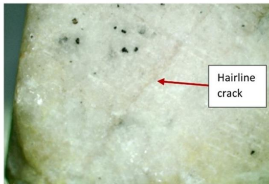
Figure 3. Hairline crack as observed in marble during the experiment
