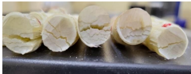
Figure 5. Failure mode of GFRP bars in horizontal shear
