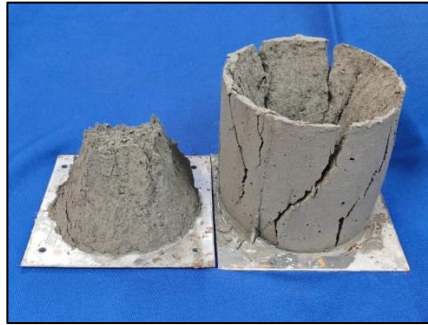
Figure 2. Failure modes of early age strength test
