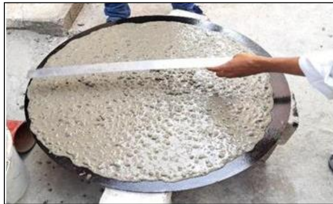
Figure 2. Slump flow test in progress
