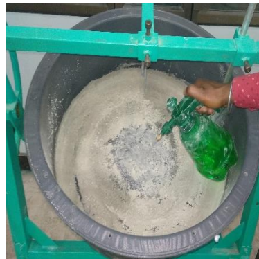
(b) Spraying of water after dry mixing
