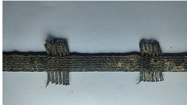
(b) SGU 200 taken out form concrete specimen after 5 years of degradation
