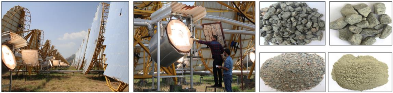
Figure 2. Demonstration of RCA Beneficiation using Concentrated Solar Energy (Prajapati et al. 2022)
