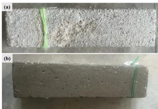
Figure 2. Acid attack consequences observed visually after a period of 150 days.
