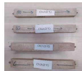
Figure 2. Mortar bars exposed to 5% sulphate for one year at 23°C
