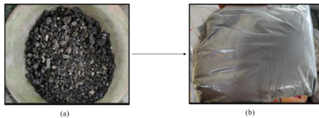
Figure 4. Slag converted to powder form using ball mill (a) Slag (b) Powdered slag
