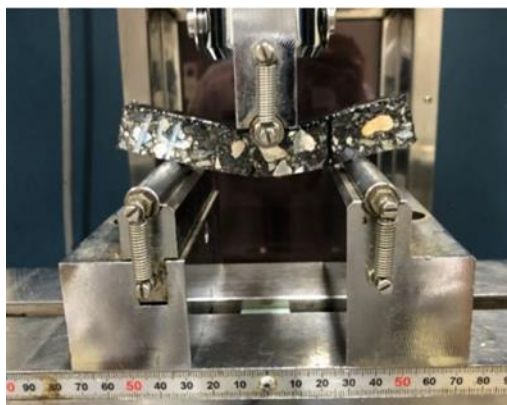
Figure 14. Static bending test situation
