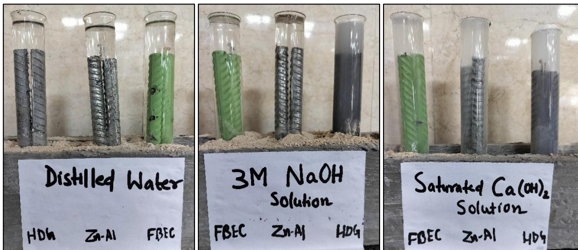
Figure 5. Samples of different coated bars are kept in various solutions for 45 days
