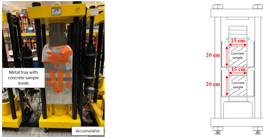
Figure 3. Experimental set-up for uniaxial creep frame
