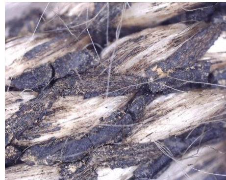
(b) GG taken out form concrete specimen after 5 years of degradation
