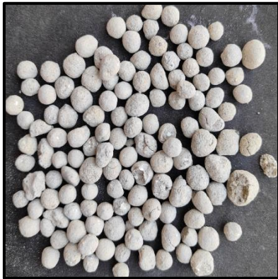
(a) Cracks were observed after 90 days
