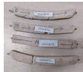
Figure 4. Mortar bars exposed to 5% sulphate for one year at 6°C
