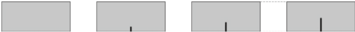
Figure 4. Boundary effect tests with the same depth of the beam and increasing initial notch size
