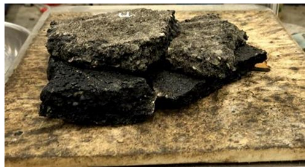
Figure 2. Base layer asphalt concrete collected
