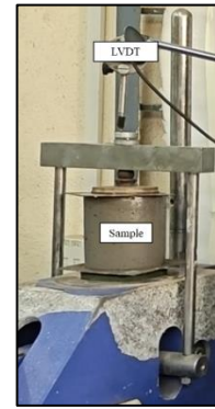
Figure 3. Early age creep test setup
