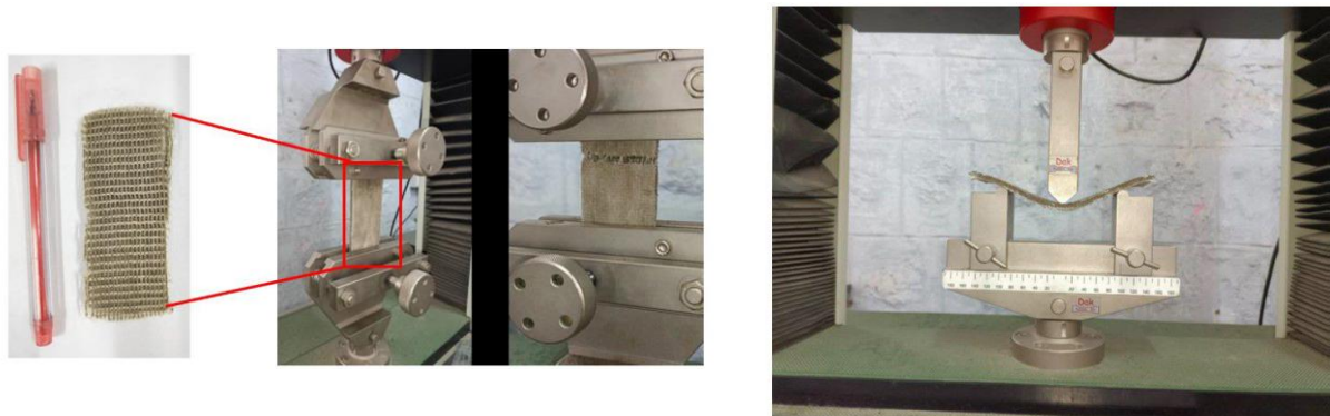
Figure 2. Geosynthetic Cementitious Composite Mats for tensile and flexural strength
