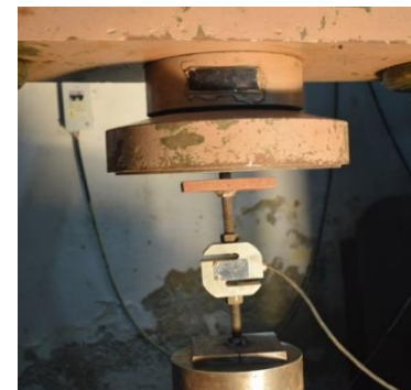
(f) Test setup for finding single aggregate crushing strength
